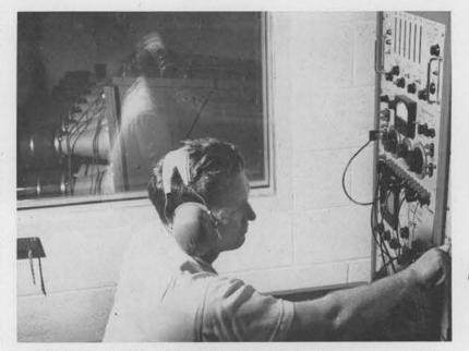
CONTROL PANEL of Sandia's Acoustic Facility in Area III is operated here by John Colburn. Through the plate glass window can be seen the 40 cubic foot test chamber and the drivers injecting sound into it. Blurred reflection is a combination of resulting vibration and the three thick plate glass windows that comprise the viewing panel. Center pane of glass rests on rubber mounts.
